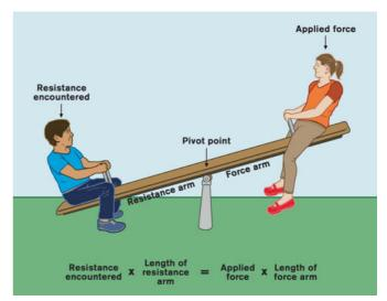
**Fig. 4-7** The law of levers relies on four variables: force applied, the length of the force arm, the resistance encountered and the length of the resistance arm. The force applied multiplied by the length of the force arm is equal to the resistance encountered multiplied by the length of the resistance arm.
